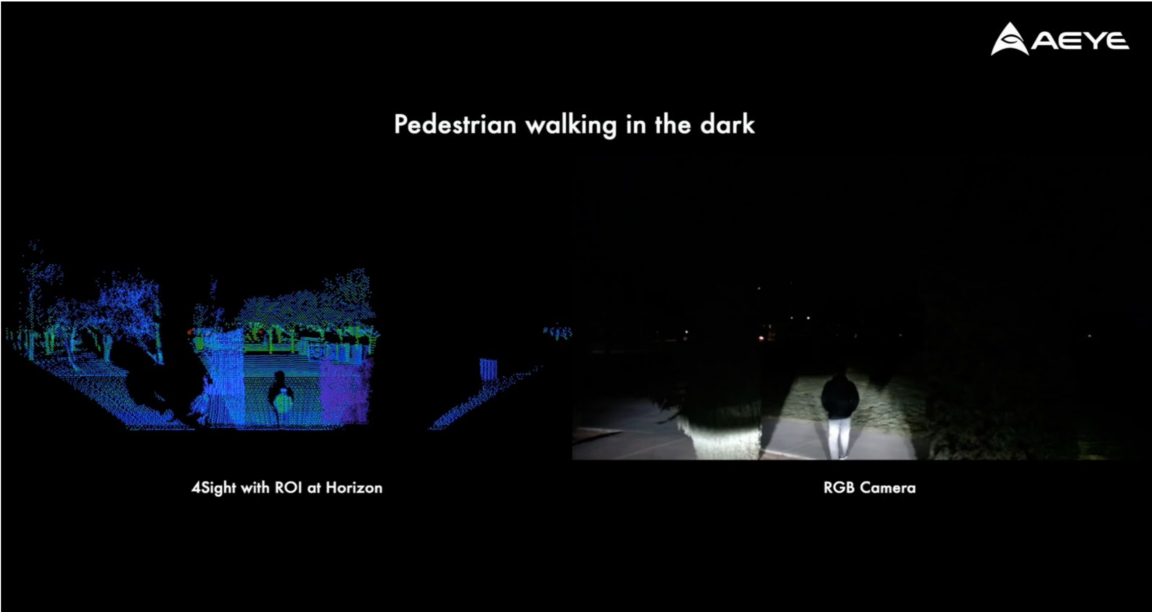
Pedestrian in low light — AEye point cloud (left) detects what the RGB camera (right) misses
